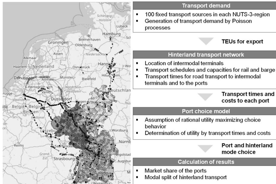
**Figure 1:** GIS map with visualization of the transport processes and modules of the simulation model
