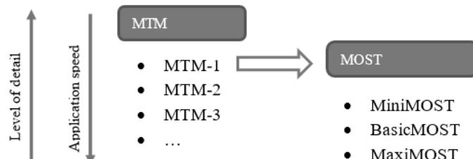
**Figure 1:** Connection between industrial work-measurement techniques and the simulation (Zandin 2003)
