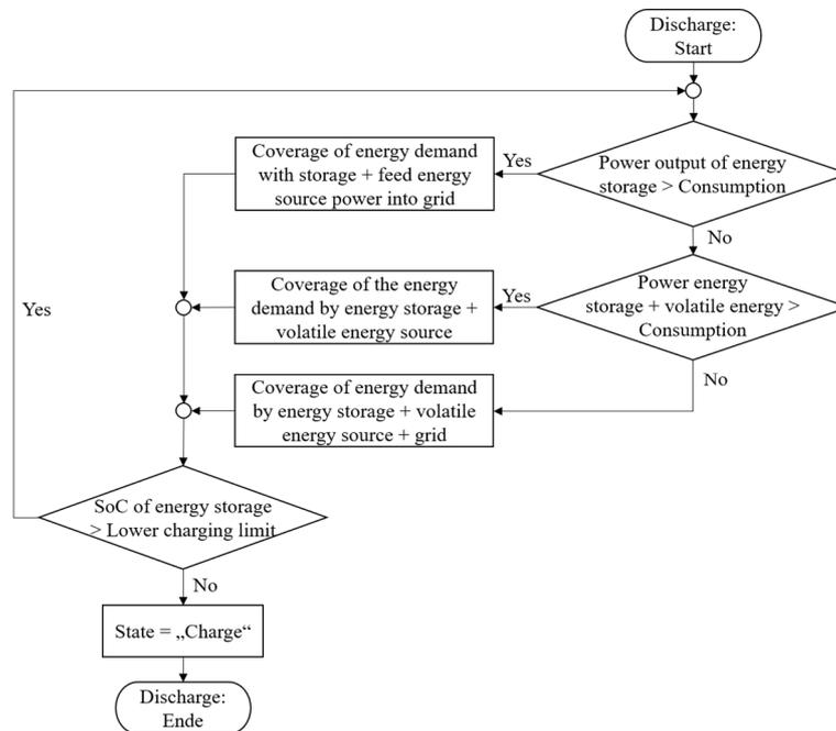
Figure 3: Control flow diagram for the discharging subprogram
