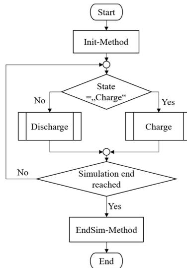
Figure 2: Control flow diagram of an energy storage device
