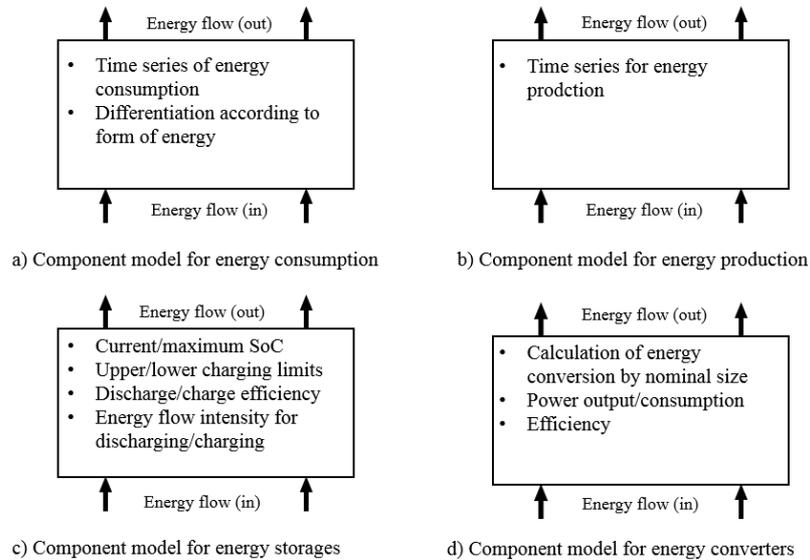
**Figure 1:** Component models for the energy flow of manufacturing systems, referring to Stoldt et al. (2017)
