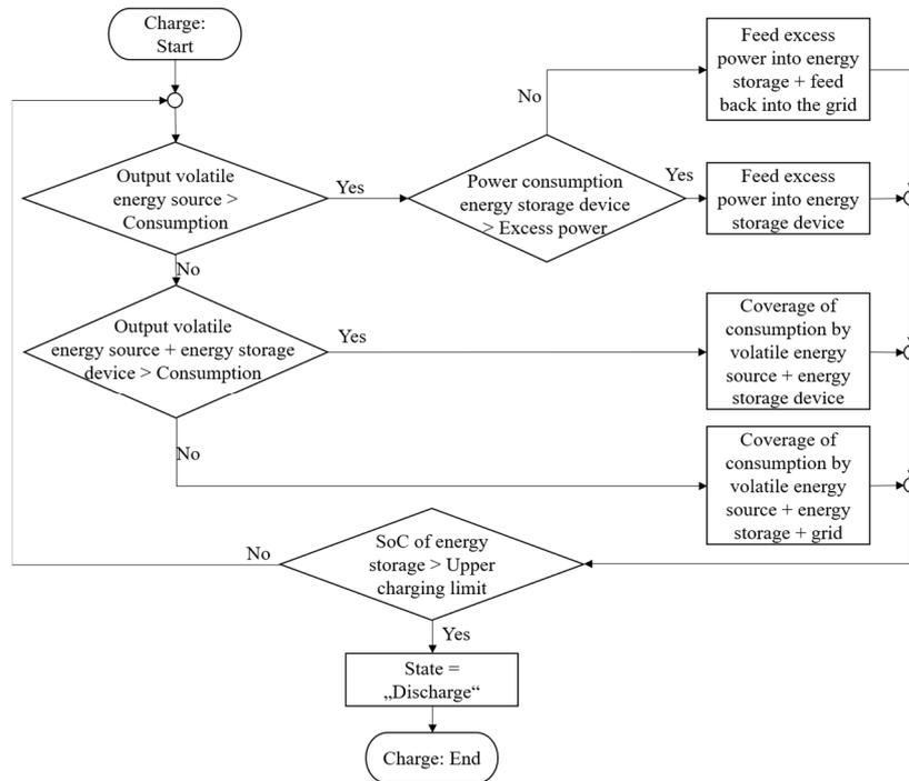
Figure 4: Control flow diagram for the charging subprogram
